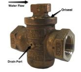
These can be a potential cross-connection if the stop and waste valve is installed below the ground surface; the water (including any contaminants, such as chemicals, dirt, bacteria, fertilizer, etc.) can pool up and then enter your internal plumbing and potentially the drinking water system through the valve when it is opened back up. The California Plumbing Code and the District requires that "Combination stop-and-waste valves...shall not be installed underground."
